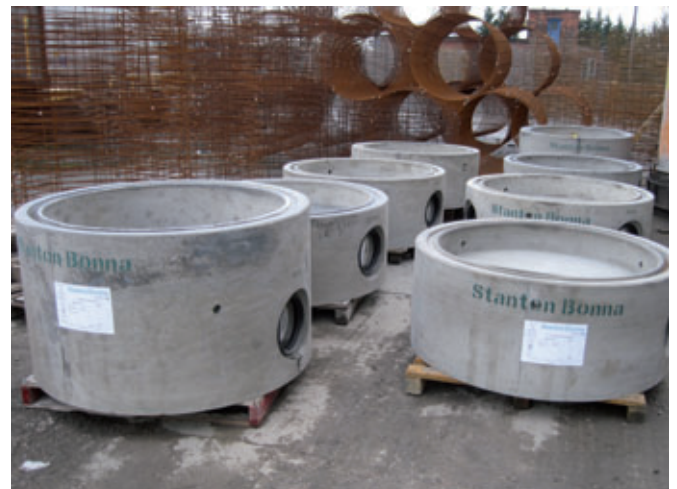
Immediately after demoulding, the manhole bases are loaded onto pallets at Stanton Bonna
