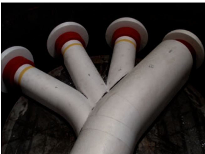
There are no limits in terms of planning freedom – all negative channel mouldings can be individually adjusted.
