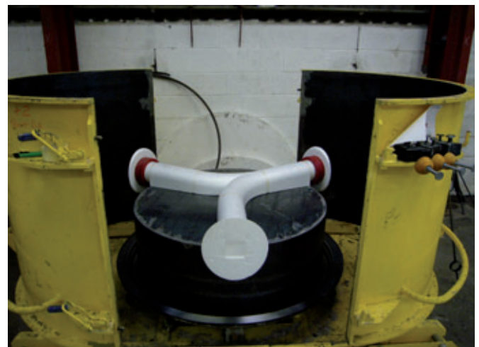
The EPS channel parts are positioned in steel moulds where they are then cast using self-compacting concrete.
