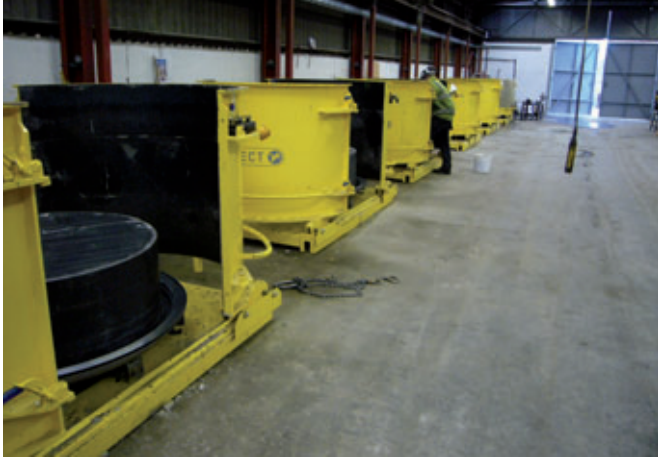
CPM manufactures monolithic Perfect manhole bases in a dedicated production hall.
