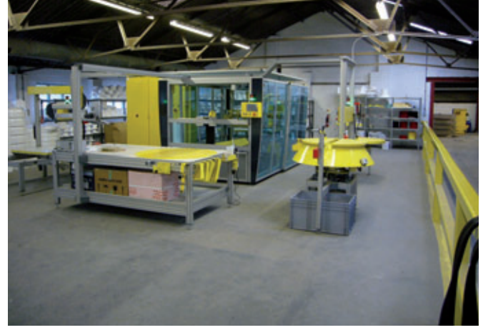
Hot wire saw technology provides simple methods in the manufacturing of individual manhole bases.
