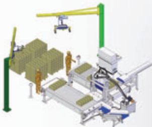
Splitting line with rotation crane
