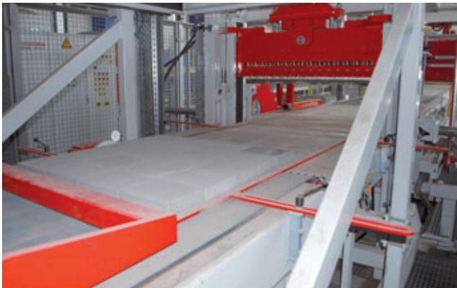
The layer is pushed under the splitting machine in rows
