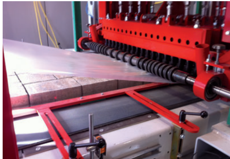
Untreated products at the intake to the aging plant; the synchronously running film protects the product surfaces against damage during the aging process.
