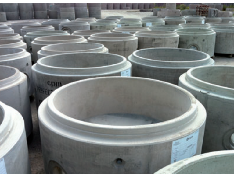
Perfect manhole bases in the loading area at the CPM site in Staffordshire
