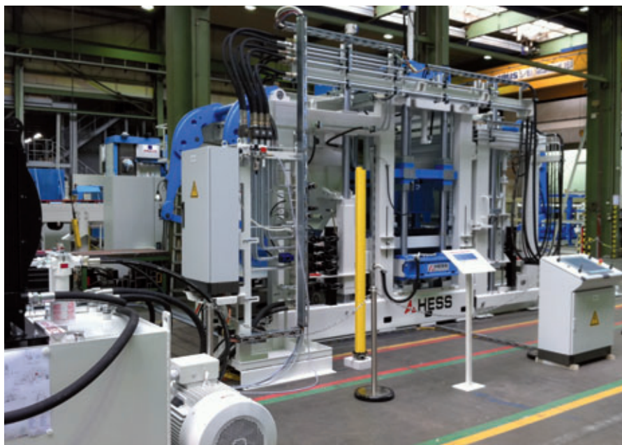
As an entry-level machine, the new RH 1400-3 VA concrete block making machine is intended to pave the way for future customers of Hess's large pallet machines
