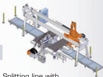
Splitting line with automatic grippers
