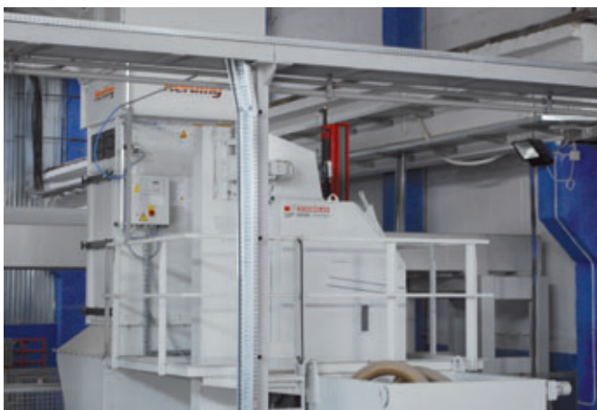
Blasting plant with sintered lamella filter
