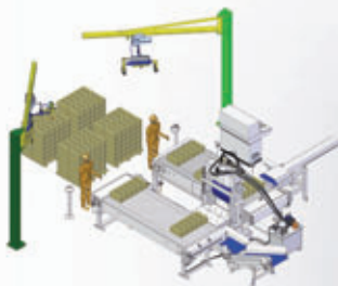
Splitting line with rotation crane
