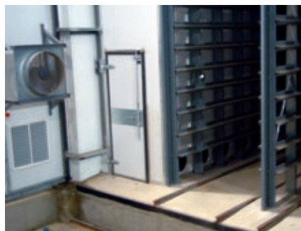
Air circulation system for optimum hardening of the products
