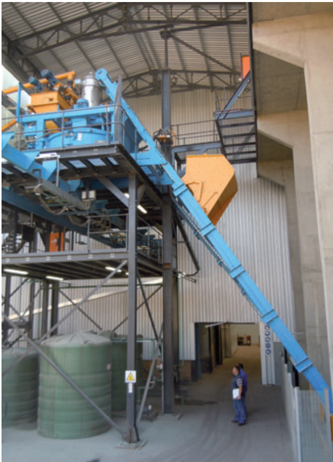
Mixer frame with Masa PH 1500/2250 and PH 200/300 horizontal compulsory mixers
