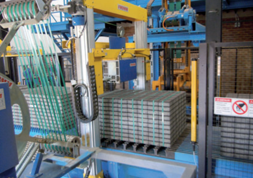
Lift and carry packet conveyor with station for vertical strapping without transport pallets
