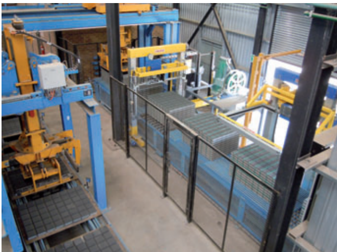
Return transport with 4-sided centring and packet transport
