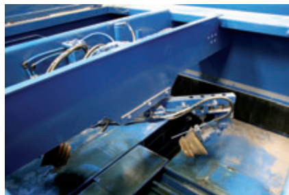
Sponges for oiling the pallets apply the oil extremely efficiently
