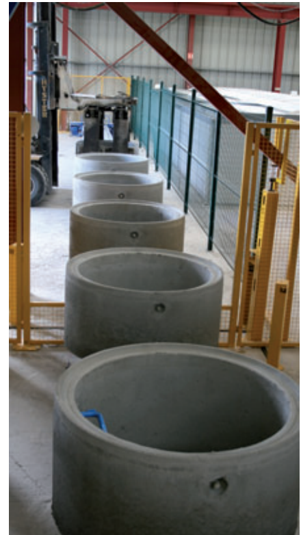
Transfer to the product conveyor belt. The concrete components leave the production hall in the next shift
