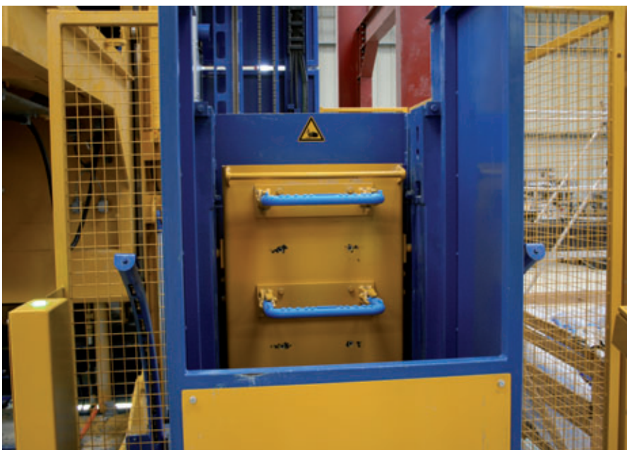
The automatic unit for fitting the moulds with step-rings is called the Stepmaster
