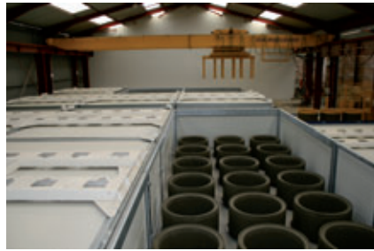
The hardened manhole rings shortly before removal by the crane robot
