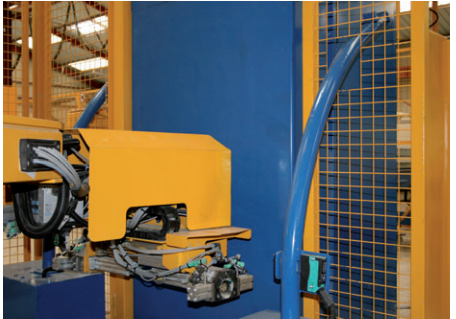
The robot fully-automatically takes two anchors and positions them into the mould
