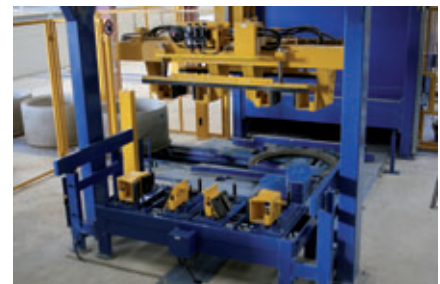
The latest development from Schlüsselbauer: the quick change unit for grippers
