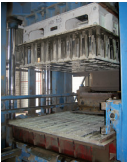
Foresight Cement Industries L.L.C. produces the 8" hollow block on a Masa XL 9.2
