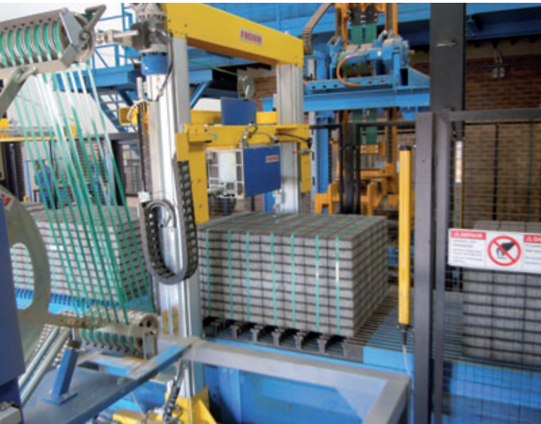
Lift and carry packet conveyor with station for vertical strapping without transport pallets
