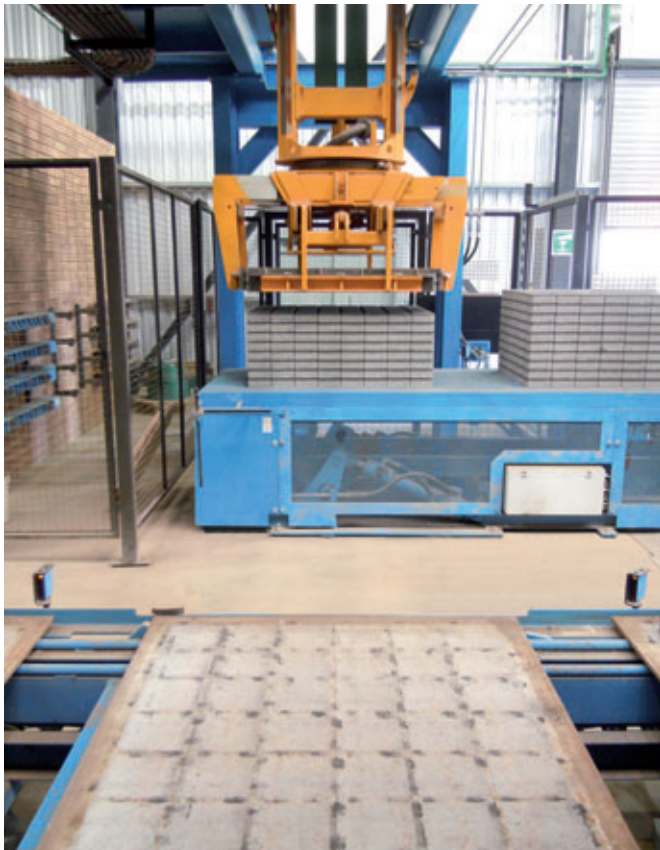
Packet assembler with servo clamp
