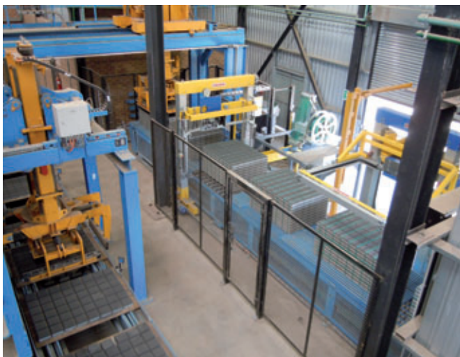
Return transport with 4-sided centring and packet transport
