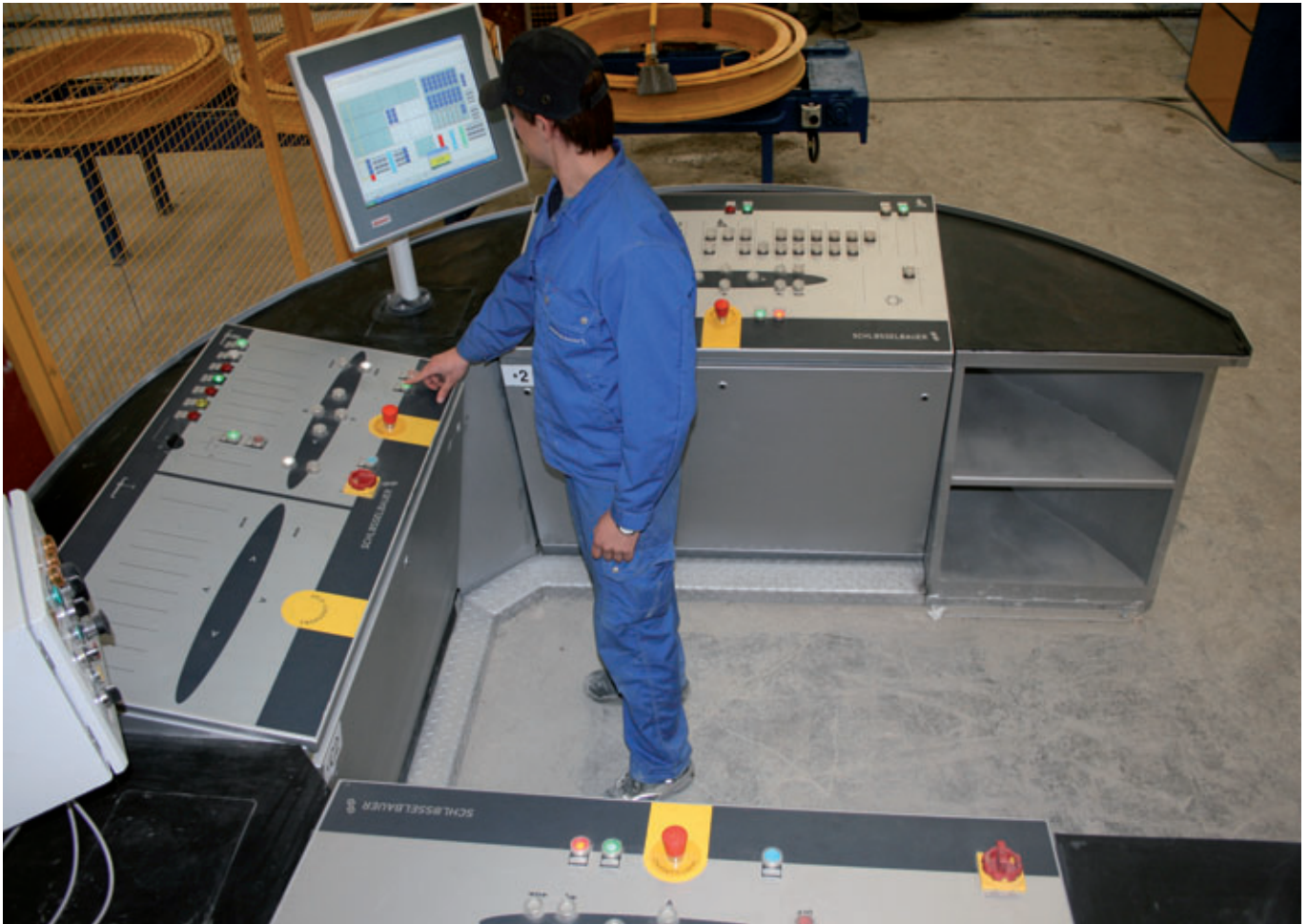
All the work sequences between the concrete mixer and removal of the products are so highly automated that one operator looks after them all.
