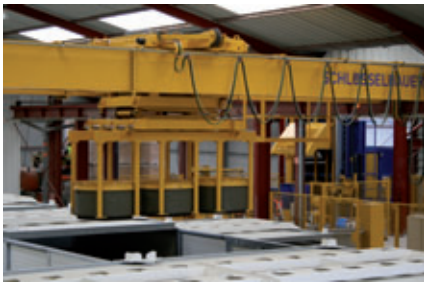
Storing the fresh manhole rings in the kilns
