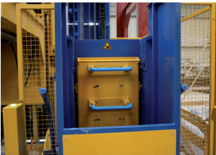
The automatic unit for fitting the moulds with steprungs is called the Stepmaster
