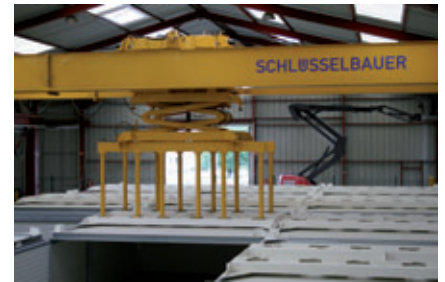
The rotating gripper bars allow the cover sections to be moved without the need to change tools
