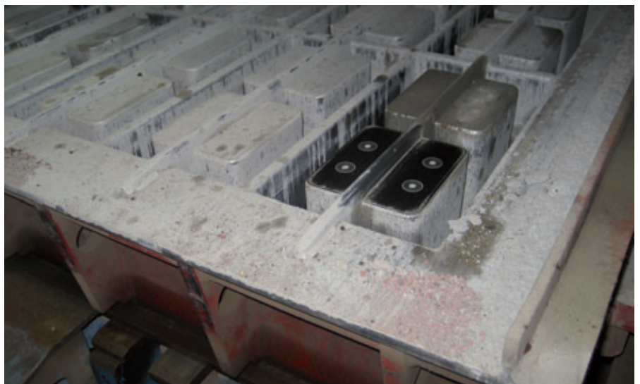
Bolted, case-hardened single cores have proven themselves in practice.
