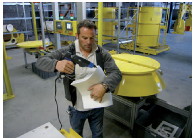
The channel sections are cut with hot wire and the negative channels are put together within a few minutes.
