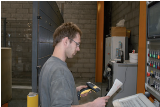
Scanning in the barcode activates the milling process
