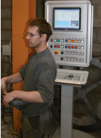
The milling speed can be controlled via remote control
