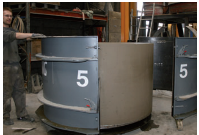
The formwork can already be stripped from the concrete monoliths after a few hours
