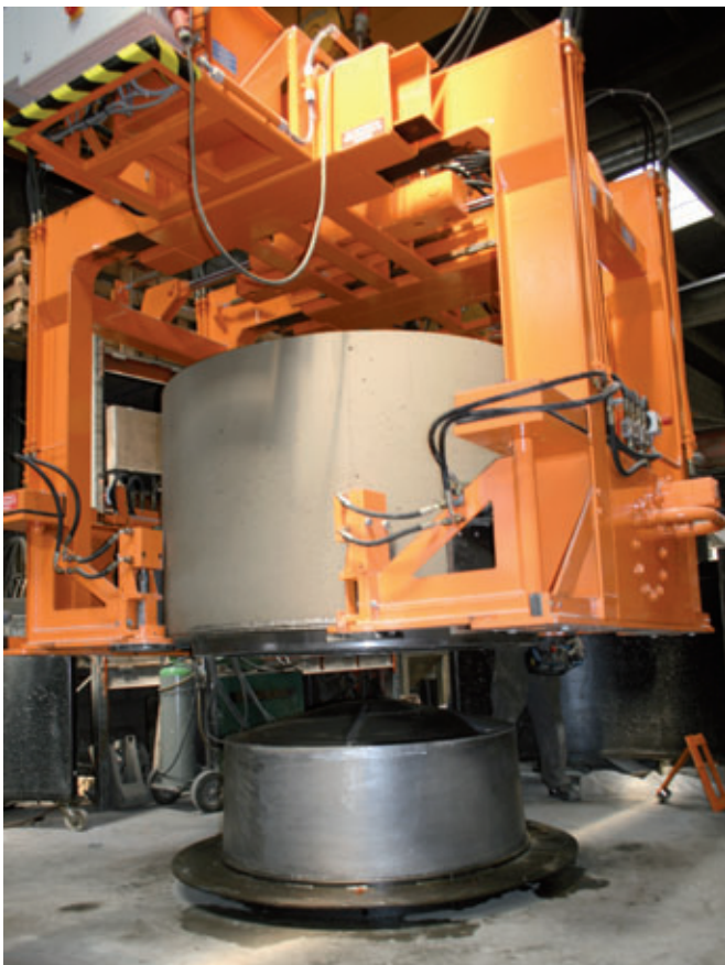
The stripped concrete element is carried on a steel pallet
