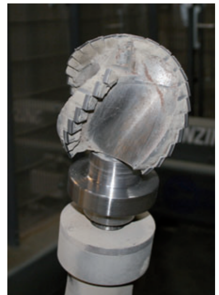
Milling head for cutting the channel
