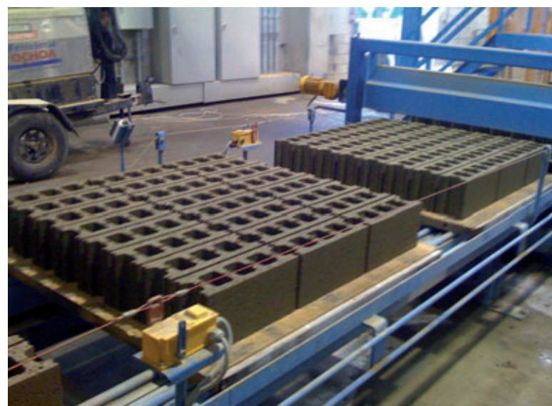
6 inch 3 cored block during production
