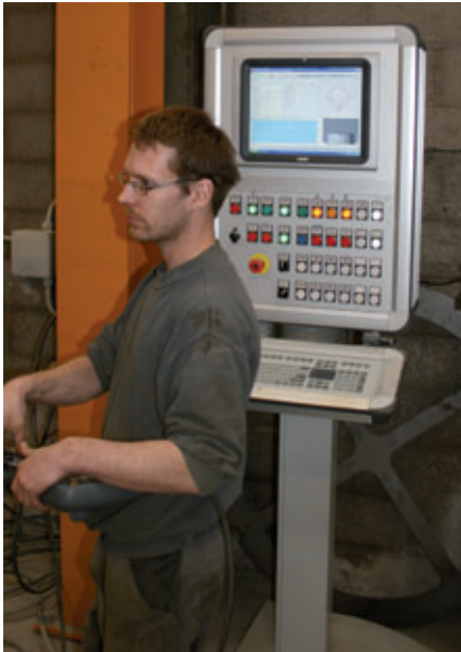
The milling speed can be controlled via remote control
