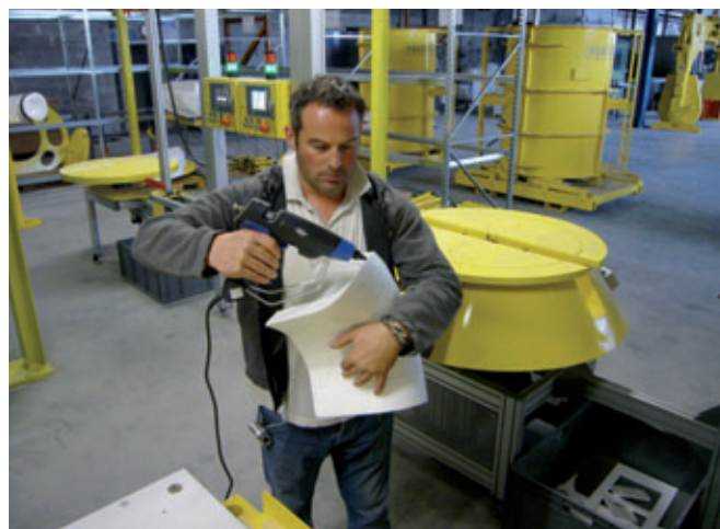
The channel sections are cut with hot wire and the negative channels are put together within a few minutes.
