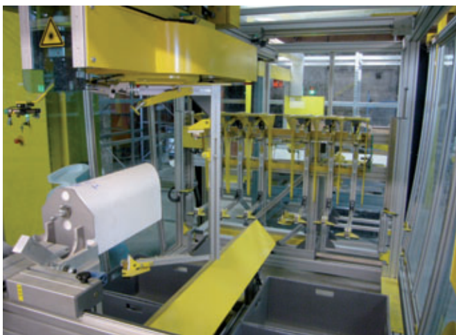
The channel sections are cut with hot wire and the negative channels are put together within a few minutes.
