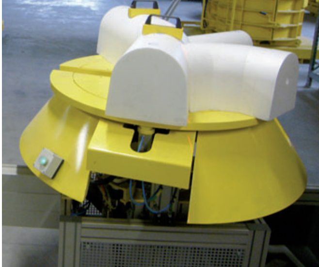
At VMC hot wire cutting is used to cut the material-saving EPS-mould parts to suit your project requirements; the picture shows the saw for shaping the berms.
