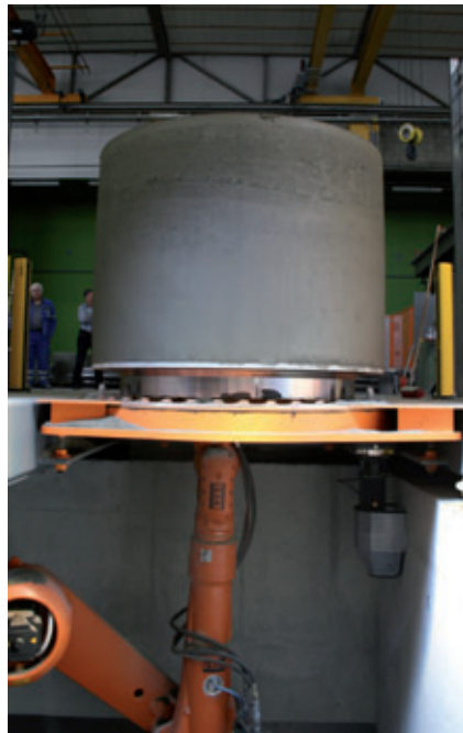
Milling a drainage channel
