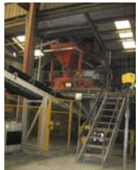
Mieszalnik 1,7 m 3 firmy ACT (Advanced Concrete Technology) .
