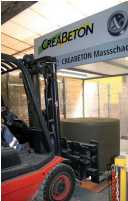
Setting down a concrete manhole blank on the clamping ring in the work bay
