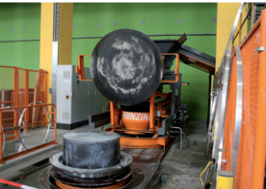
First, the steel pallet and support cap are positioned in the Atlas plant
