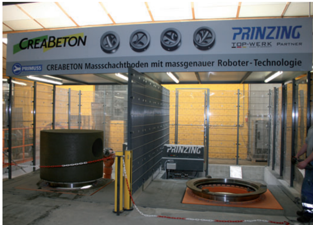
Primuss milling bay with two work places
