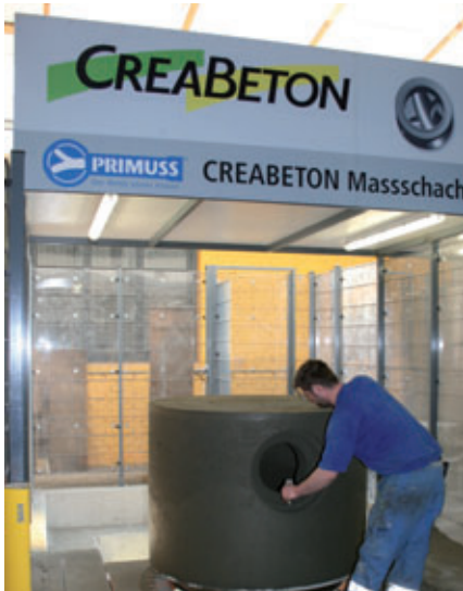
Pipe connections are swept out at the end
