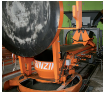
Dosing shutters control the flow of concrete
