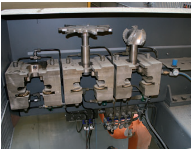
The two-part tool storage unit offers mountings for a total of six milling heads
