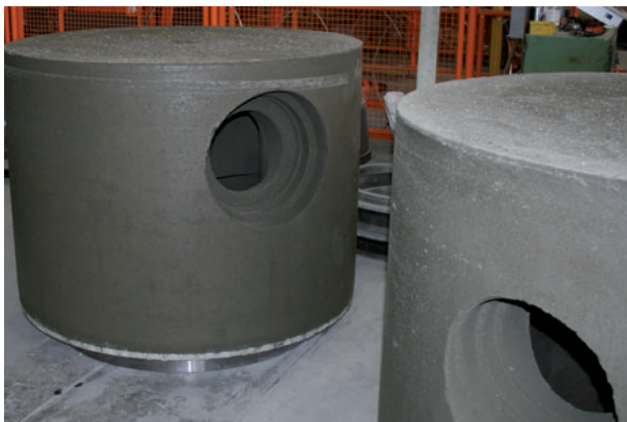
Milled manhole monoliths in the storage area for furthering hardening
