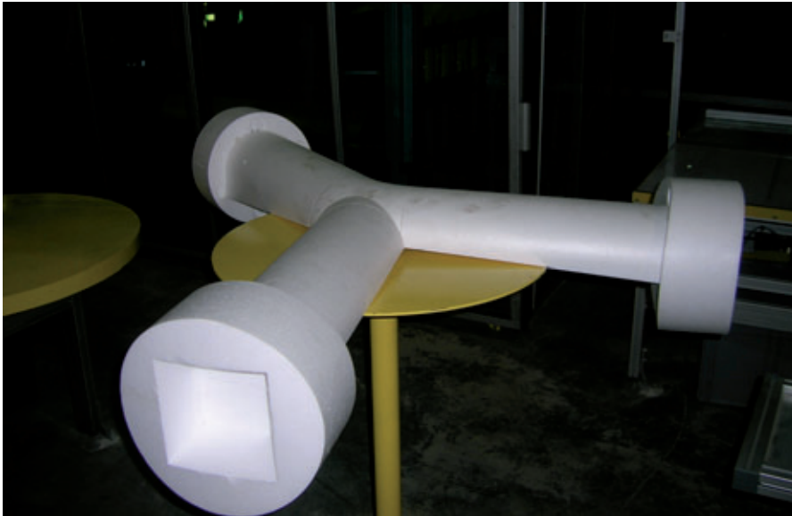
The completed construction of a negative mould piece.
