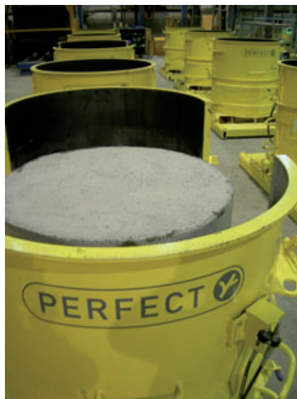
Perfect moulds installed in a stationary arrangement at Con Cast Pipe
