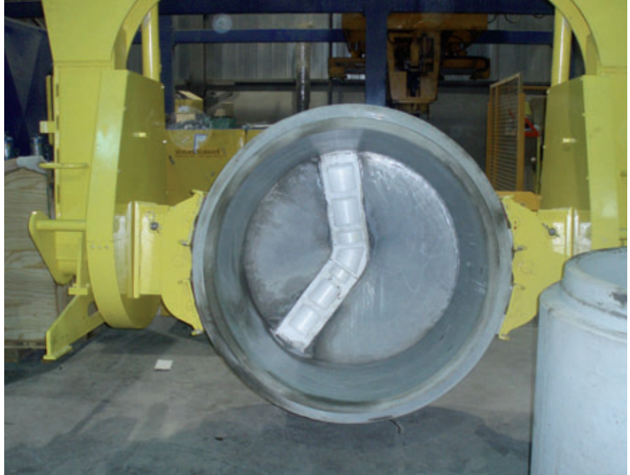
Demoulded products are turned in their assembly position.
