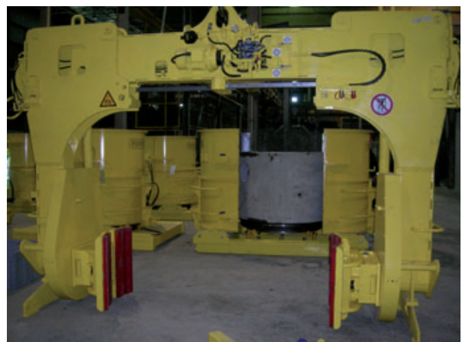
Manipulation of cured products by an existing overhead crane and a turning devise.
