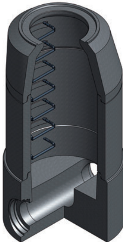
Manhole with cone
