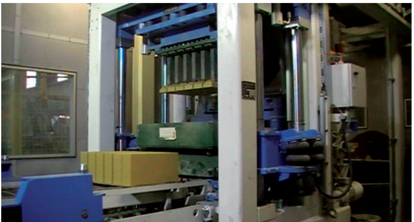
Concrete block machine
