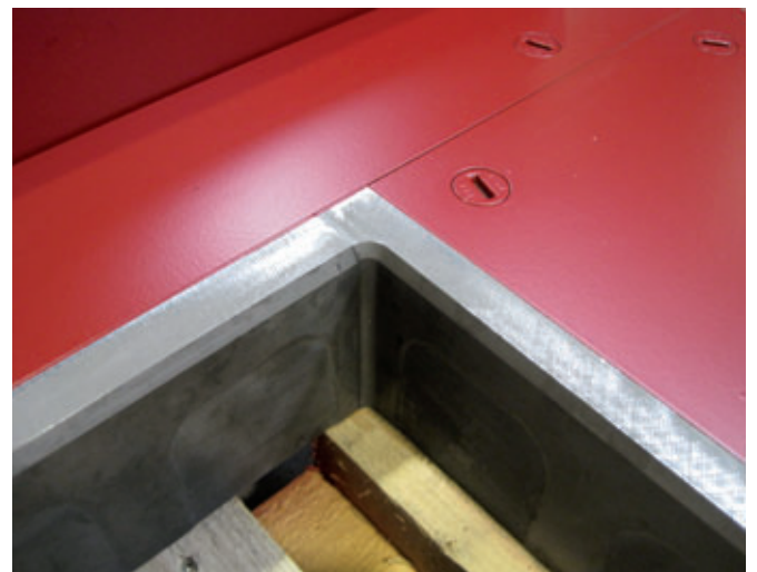
Fig. 5: Mould corner with innovative single walls in standard hardness 68 HRC
