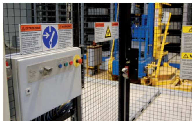
Safety interlock systems for the safe opening of doors – in combination with local release terminals for plant safety
