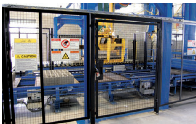
Signs and other safety-relevant notices on plant components are decisive for the employees' safety understanding and sensitise them to possible sources of danger.
