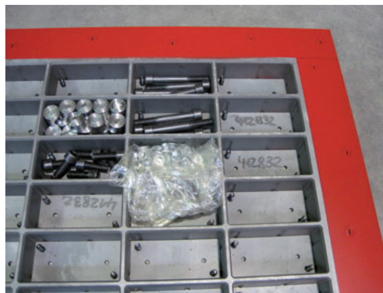
Fig. 2: 'Moduline2' mould lower part with separately delivered pressure plates and mounting kit for bolted flanges
