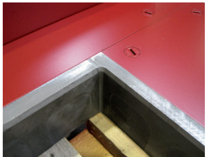
Fig. 5: Mould corner with innovative single walls in standard hardness 68 HRC
