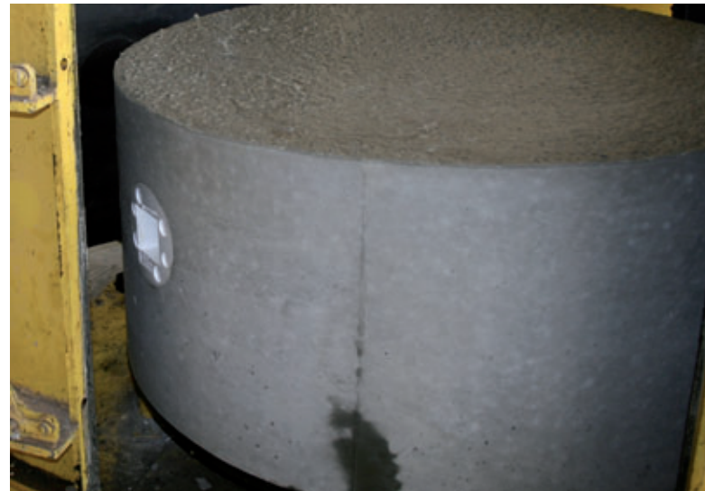
Hardened manhole base after the mould is opened
