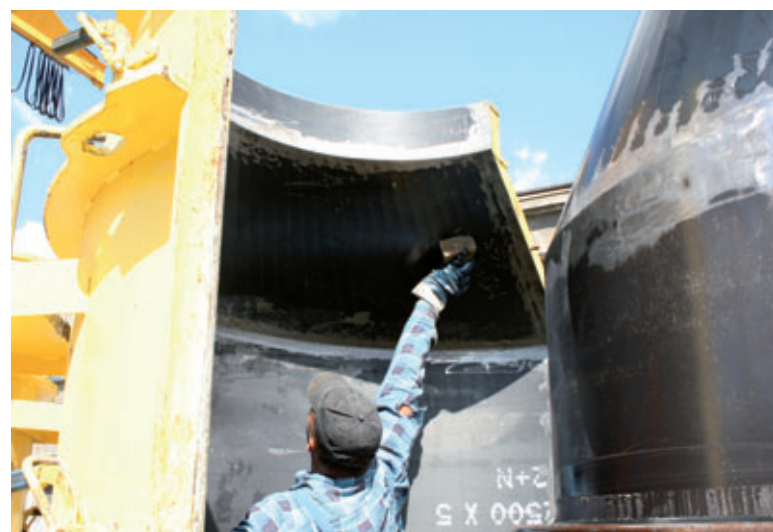
Greasing the formwork surfaces with Ortolan SEP 791 release paste from MC Bauchemie
