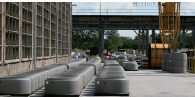
Kaprin produces manhole rings with the Schlüsselbauer Precise manhole ring machine installed in 1997
