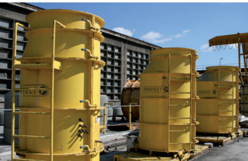
The three new moulds for up to 2,350 mm high concrete manhole cones with nominal widths of 1,000, 1,200 and 1,500 mm
