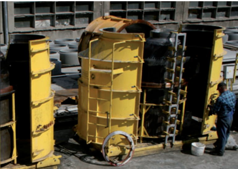
A special template is hung on the mould core for the exact setting of the bushings for the steps
