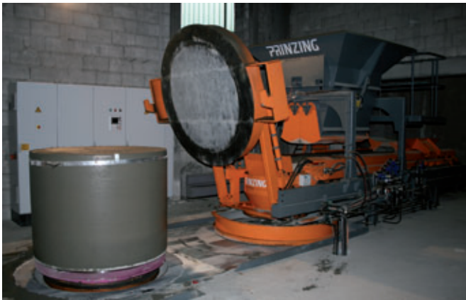
The concrete manhole monoliths are produced by the proven Atlas machine
