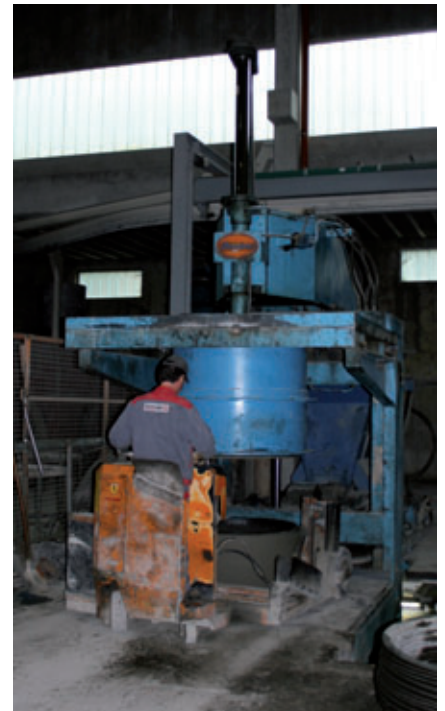
Prinzing machine for manhole ring production, manufactured in 1982
