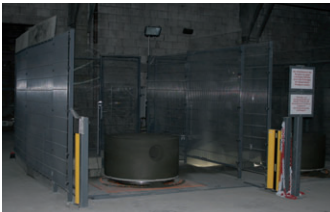
The Primuss milling station has two floor-level machining stations
