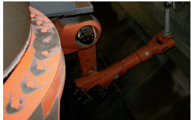
The pit under the machining stations serves as the movement area for the milling robot
