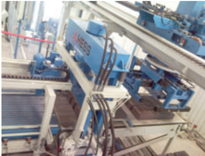
Block blanks are brought to the servo-driven packaging machine on a transport pallet; the packaging machine takes one complete layer at a time and sets it onto the splitter line
