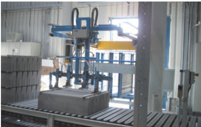
Transfer carriage for stacks of boards between the wet side and dry side or intermediate board storage unit
