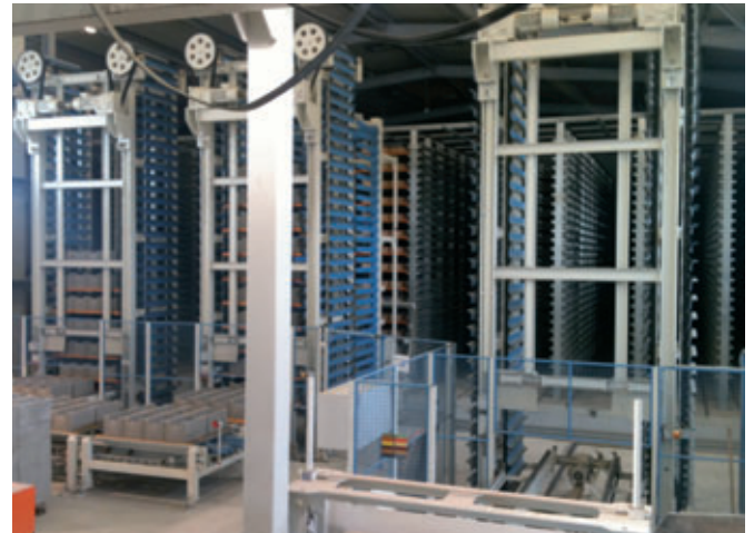
On the left, the two destackers and on the right, the stacker
