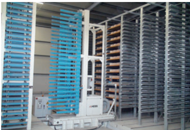
Finger car with 26 levels and rotating device
