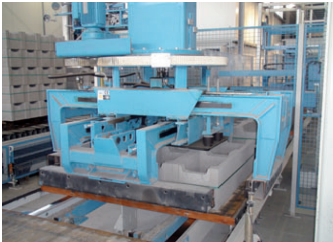
Packaging machine with servo and belt drives
