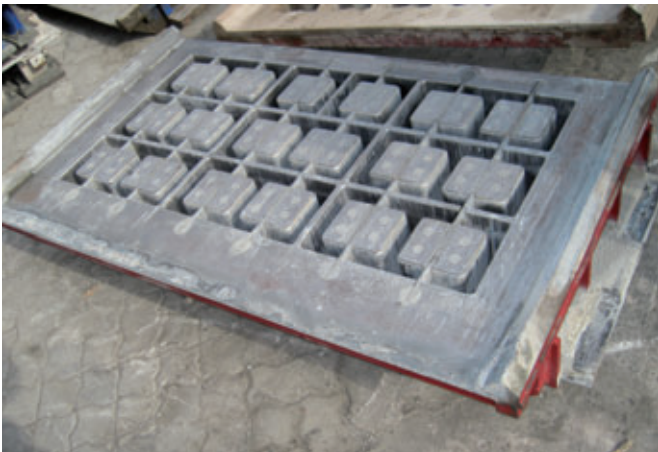
No visible wear could be found at the hollow block mould with »carbo™« – hardness after over 50,000 production cycles
