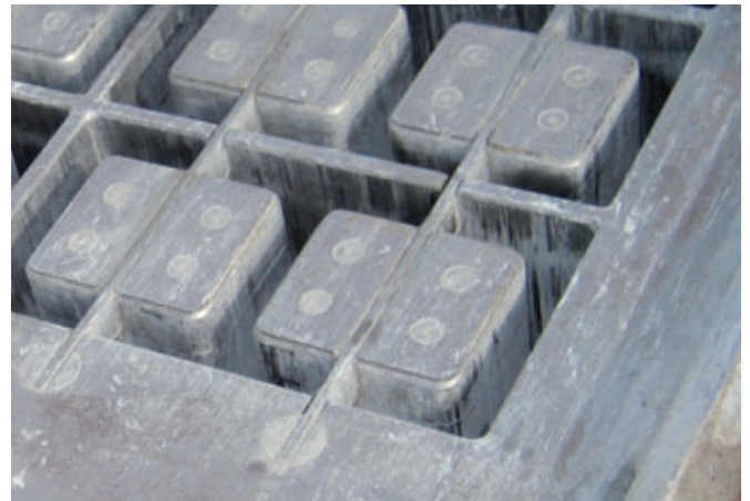
Sturdy bolted connections on the core holder bar allow the exact fitting of the CNC-machined, exchangeable individual cores in the cavity
