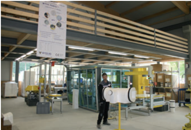
The channel sections are cut with hot-wire saws and assembled to the negative channel in the rear area of the new hall extension. The store for the EPS hard foam blanks is located in the level above this area.
