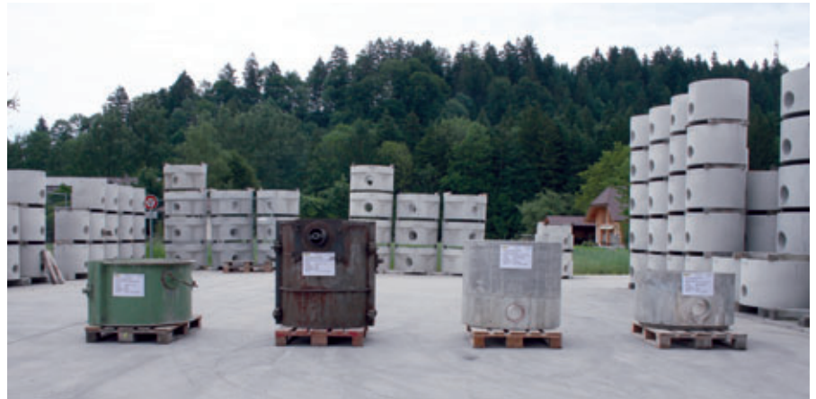
As part of the jubilee celebrations, visitors were shown the development in concrete manhole base construction at Wyss with models (from left to right): 1. Steel mould with built-in seal, 1994 2. first steel mould with built-in pipe connection, 1990 3. Concrete manhole from 1989, mould made of wood and plastic, PVC-seal cast in concrete 4. Concrete manhole from 1988, mould made of wood and plastic, grouted Eternit seal
