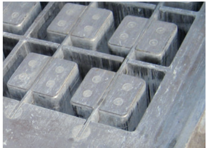
Sturdy bolted connections on the core holder bar allow the exact fitting of the CNC-machined, exchangeable individual cores in the cavity
