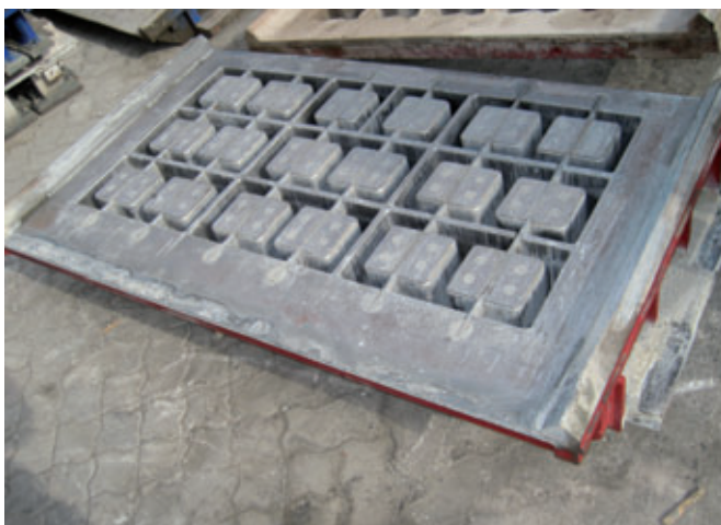
No visible wear could be found at the hollow block mould with »carbo™« – hardness after over 50,000 production cycles
