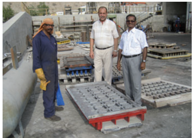
The innovative bolted connection of the core subassemblies makes mould maintenance and service much easier for National Tiles & Blocks Ltd. in Ras-Al-Khaimah, UAE
