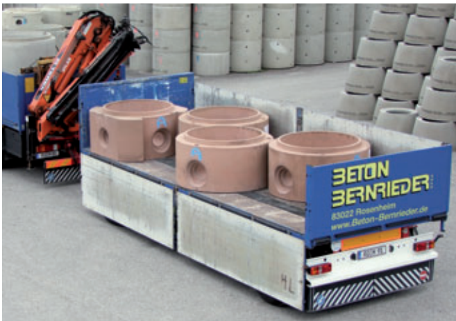
Tailor-made monolithic Perfect concrete manhole bases are produced from standard concrete C40/50 and from high-performance concrete C60/75.
