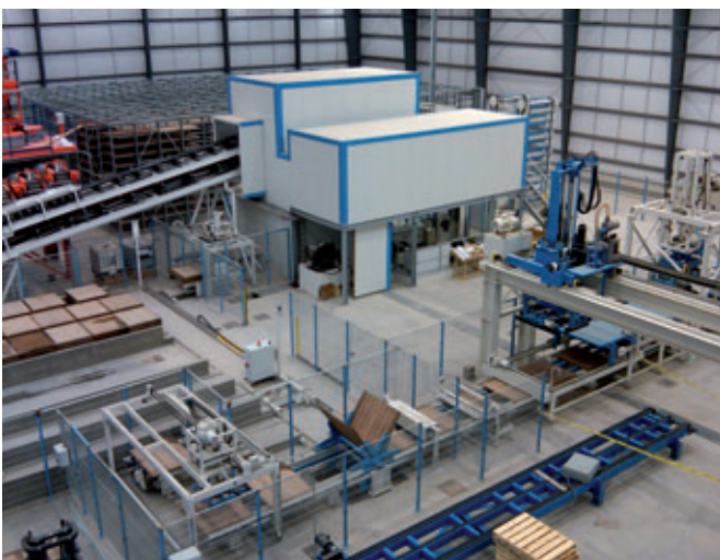
Fig. 1: The automated plant design at Sims Stone optimizes the wet side with the dry side for the best results in product quality, throughput, and unit cost.
