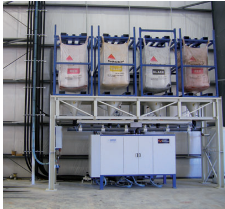
Fig. 5: An ACT Würschum COM 70-3 precision granular color pigment metering system features closed-loop pneumatic dispensing from three separate conveying vessels for a totally automatic, high output dust-free operation.
