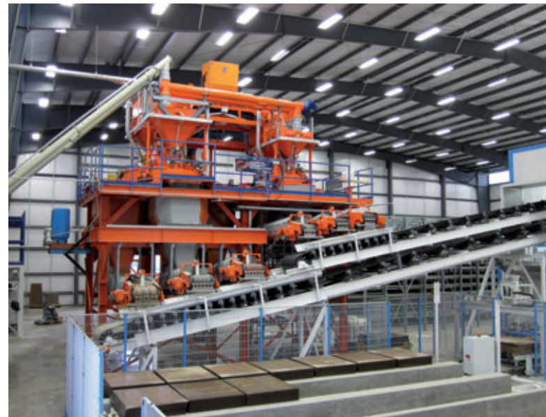
Fig. 6: The ACT MobilMat batch plant (in background) features a Twin Mixer Plant with a Wiggert HPGM 2250 and a HPGM 750 high shear mixer each feeding three concrete metering hoppers, allowing automatic mixing of three different colors for value added color-mix production of both color-thru and hard-faced paver products. The ACT MobilMat concrete batching system, equipped with the ACT HYDROMAT microwave water metering system for consistent water/cement ratio adherence, produces consistent and high quality concrete. The Hess system produces pavers and retaining walls on large steel production boards.
