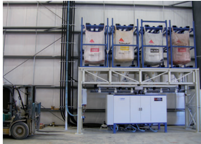
Fig. 5: An ACT Würschum COM 70-3 precision granular color pigment metering system features closed-loop pneumatic dispensing from three separate conveying vessels for a totally automatic, high output dust-free operation.
