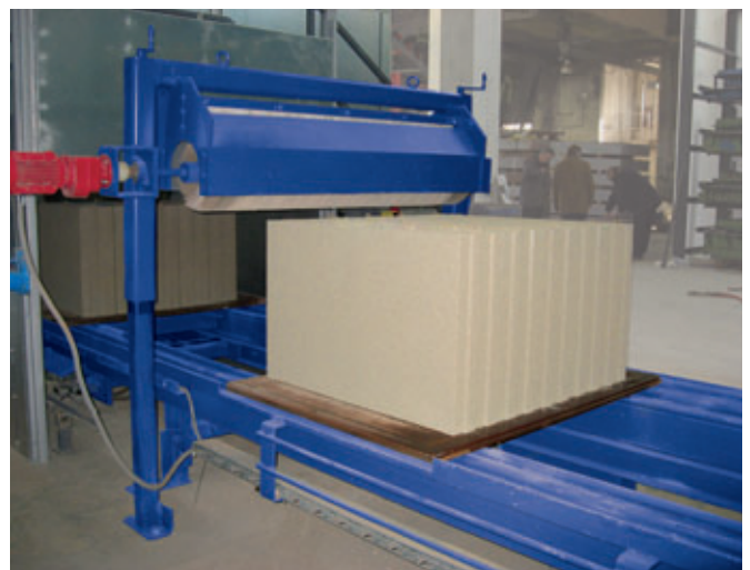
Products made on Masa XL 9.1 with aluminium vibration table, max. product size manufactured at present 1000 x 240 x 623 mm (length x width x height)
