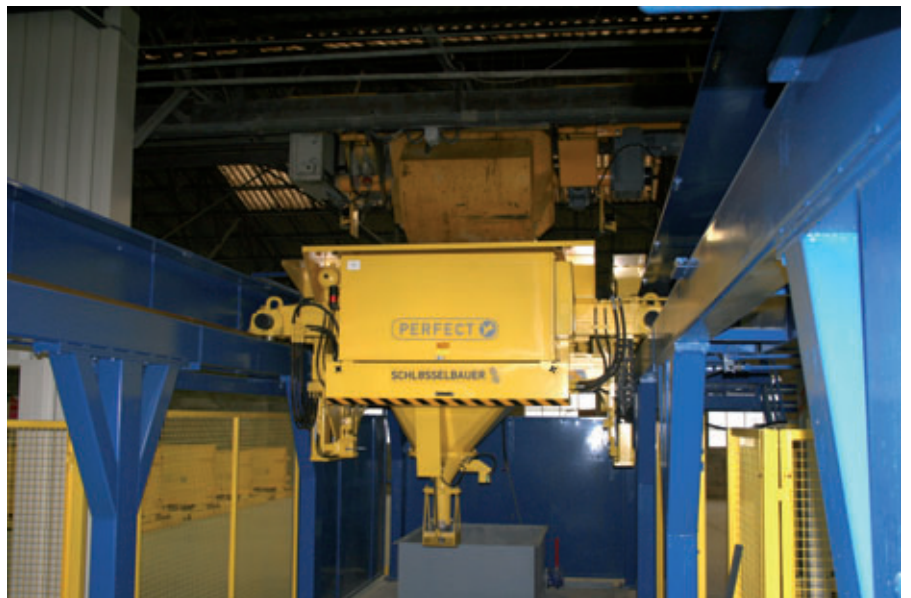
The bucket conveyor in the nearby hall also provides the Perfect production system with SVB
