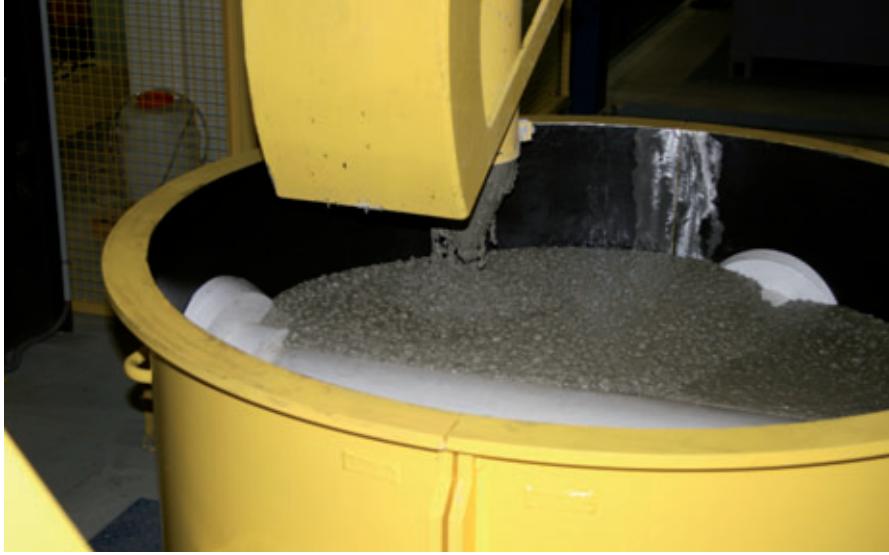
The casting head on the station ensures the mould is properly filled
