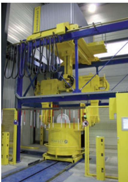
The hardened manhole bases are removed from the open mould with the gripper of the crane rail....
