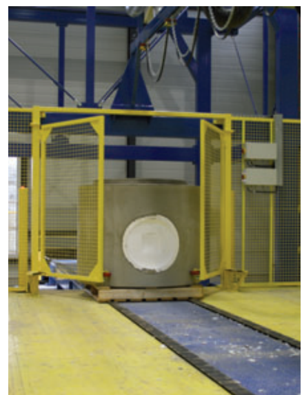
...and set onto the conveyor belt to the last processing station, in which the EPS mould bodies are removed from the manhole bases.
