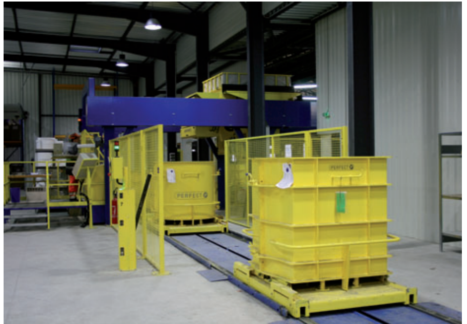
The prepared moulds drive automatically into the casting station
