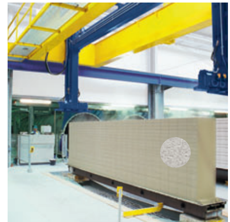
Plants for the manufacture of Aerated Concrete Blocks
