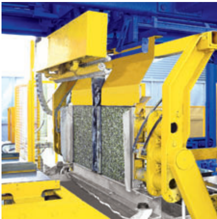
Plants for the manufacture of Concrete Slabs
