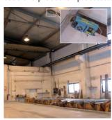
By means of a computer-controlled laser system and suitable software flow charts and measuring points can be transferred to assembly surfaces.
