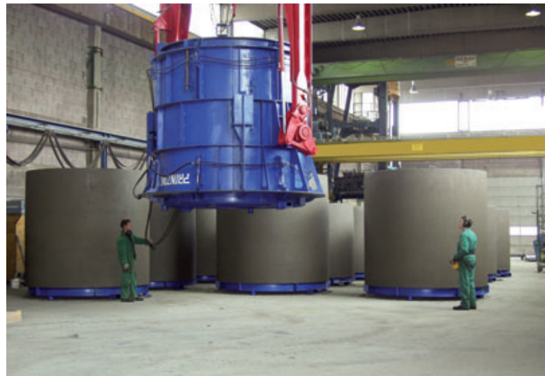
Container manufacturing with integrated cover
