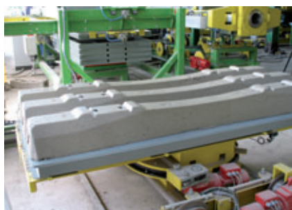
Concrete railway sleeper production with Rimac systems
