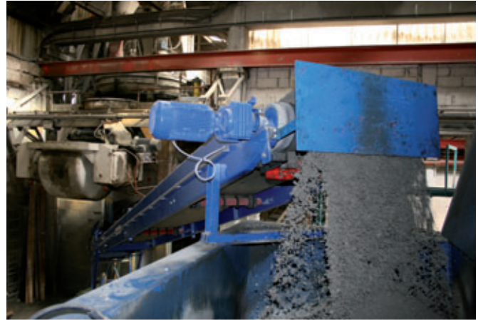
The Magic 1501 is supplied with concrete from the mixers of Frühwald's existing concrete production
