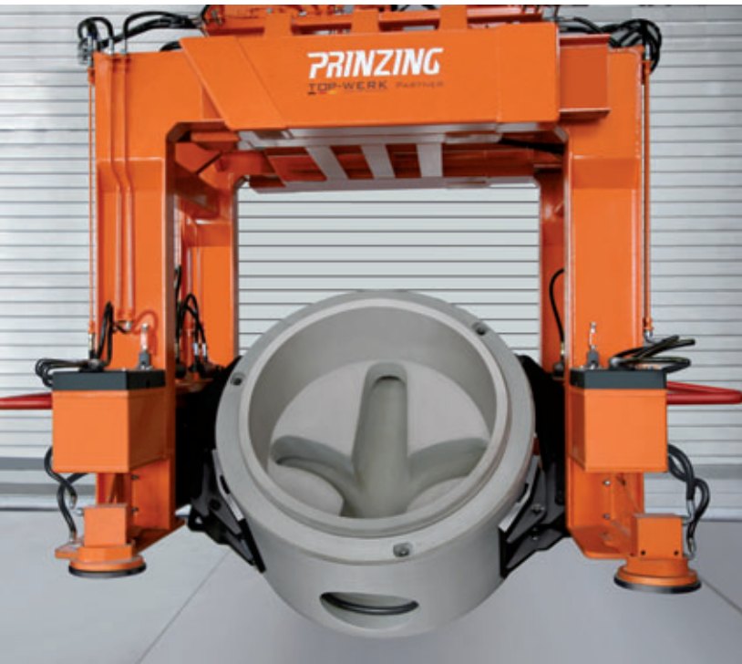
Right after the milling stage, the manhole bases are turned to their normal position
