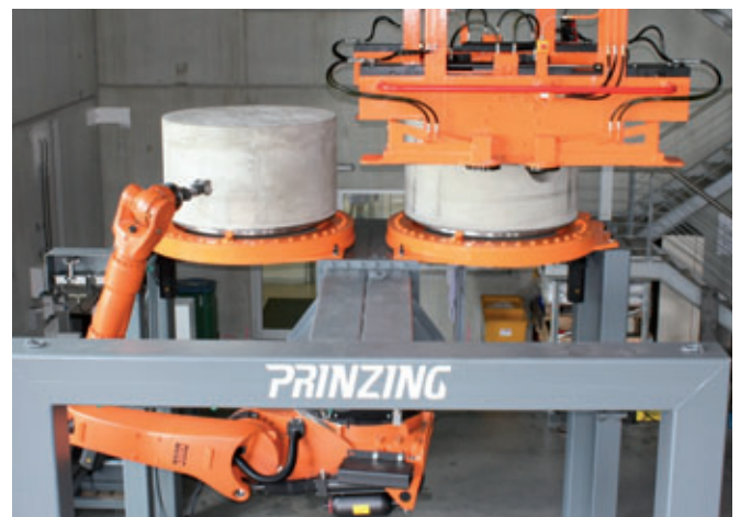
The monoliths, still resting on the steel end ring in a semi-cured state, are deposited at the milling bay and then centred with great precision
