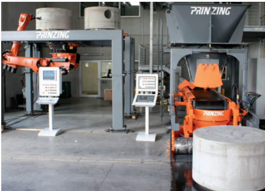
Producing monolithic manhole bases with the Primuss
