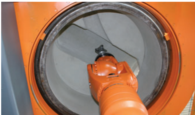
Channels are milled out from below
