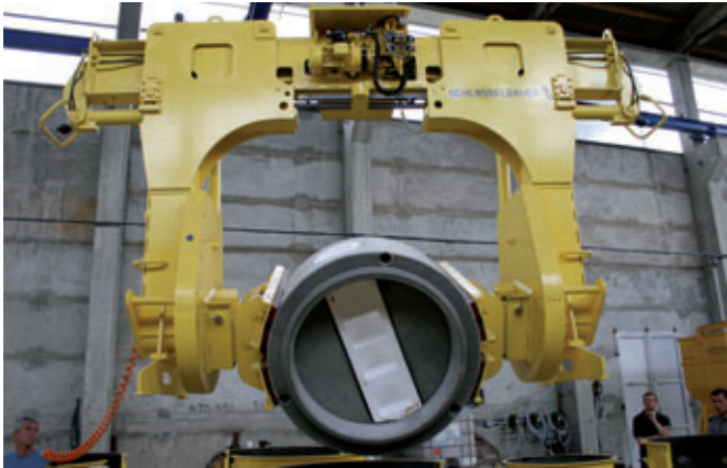
The manhole bases are grabbed with the special turning grabber and turned 180°
