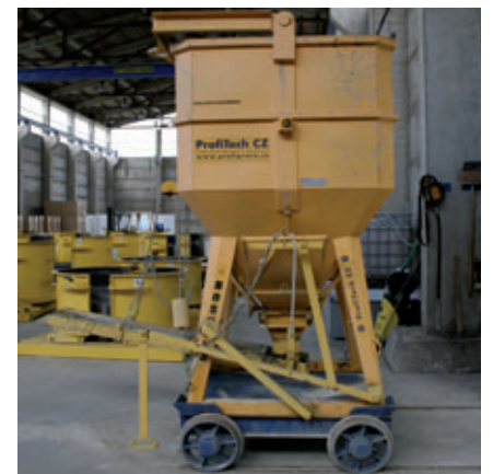
A bucket car transports the concrete at Zábajník s.r.o. from the outside area into the production building.
