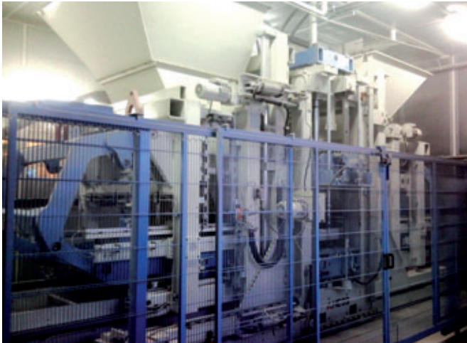
Special openings in the acoustic enclosure for feeding the Hess RH 1500-2A
