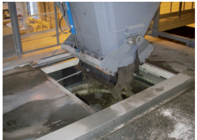
Special openings in the acoustic enclosure for feeding the Hess RH 1500-2A
