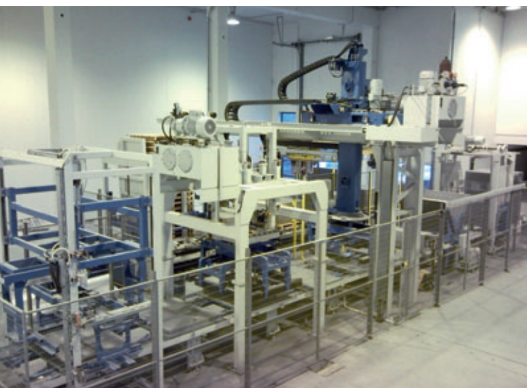
Overview of the dry side with stone releaser, stone doubler, packet assembler, board brush, board turner, board stacker and board stack transport track in the foreground; the transport pallet silo and stretch wrapping machine are in the background
