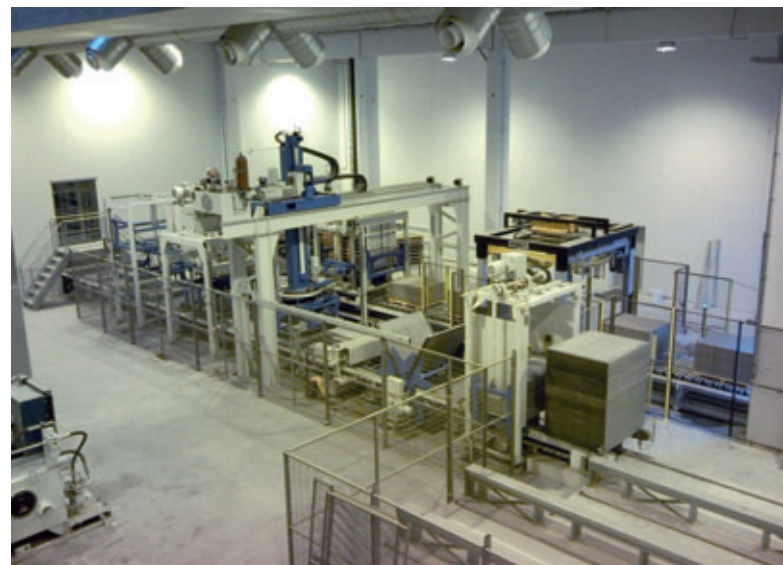
Overview of the dry side with stone releaser, stone doubler, packet assembler, board brush, board turner, board stacker and board stack transport track in the foreground; the transport pallet silo and stretch wrapping machine are in the background
