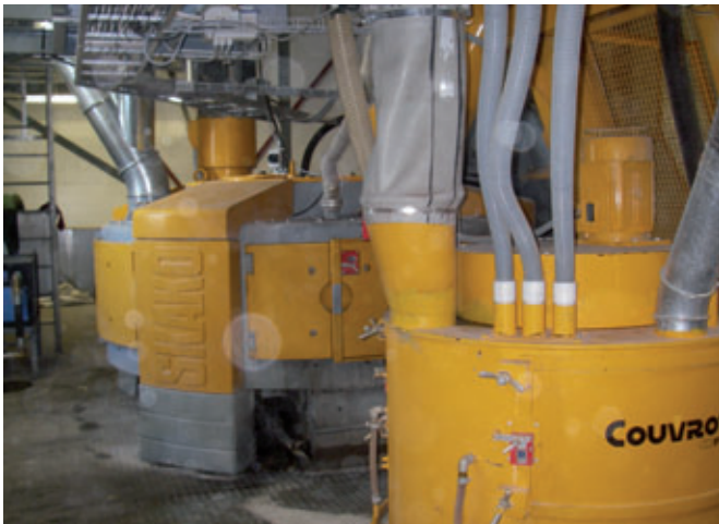
The Couvrot HTV 420 and the Skako Apollo 3000 provide the right 'mix'
