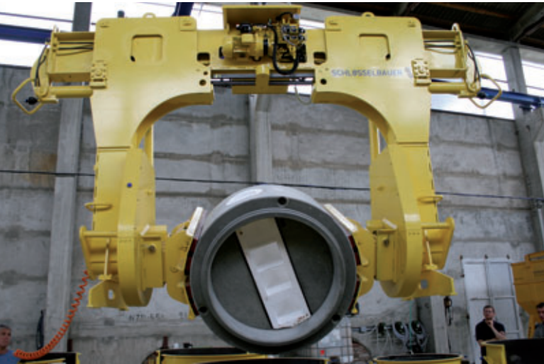
The manhole bases are grabbed with the special turning grabber and turned 180°
