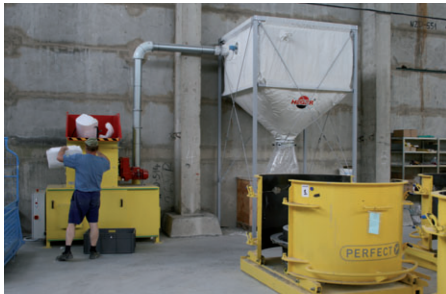
The removed EPS pieces are crushed in a shredding machine from Heger GmbH
