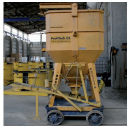
A bucket car transports the concrete at Zábajník s.r.o. from the outside area into the production building.
