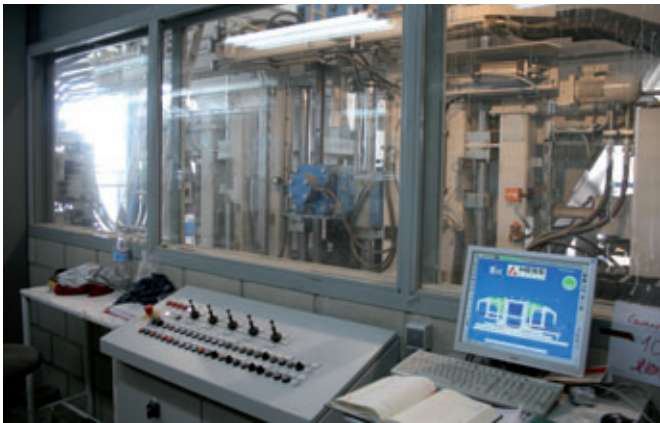
The mixer and the concrete block production can be monitored from the centrally situated control room
