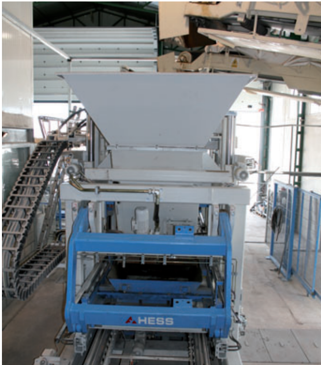
The RH1 500-2 VA concrete block making machine is fed by a conveyor belt
