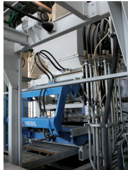
All common concrete products up to height of 400 mm can be manufactured on the RH 1500-2 VA concrete block making machine
