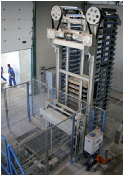
Following manufacture the product is transferred to the V-belt conveyor via a lowering device and transported to the elevator
