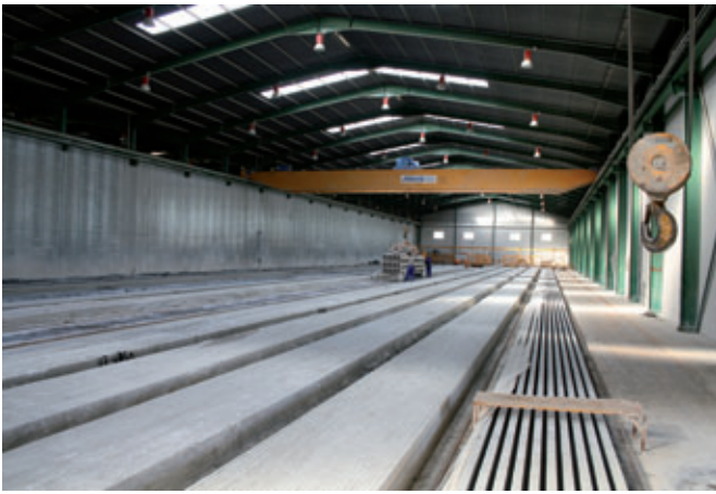
The prestressed hollow-core slabs manufactured on plants by Elematic and Prensoland are produced on a total of 14 lines, each of which is 165 m in length
