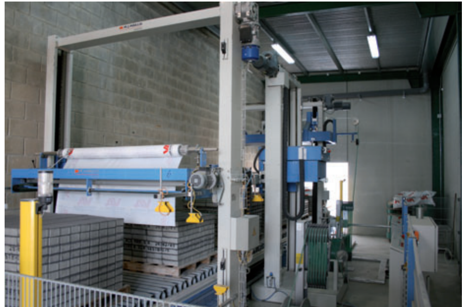
A cover sheet feeder and horizontal and vertical strapping finally ensure that the products are protected during storage and transport
