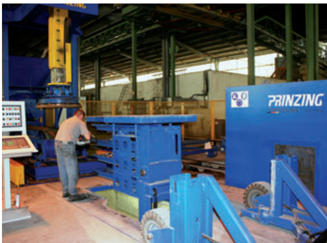
Filling up the manhole step magazine
