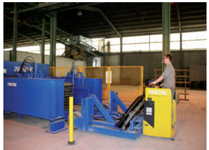
Feeding the steel pallets
