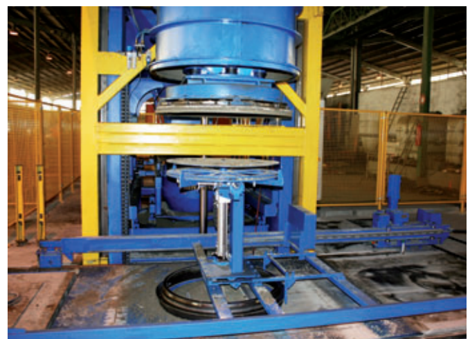
Automatic insertion of transport anchors
